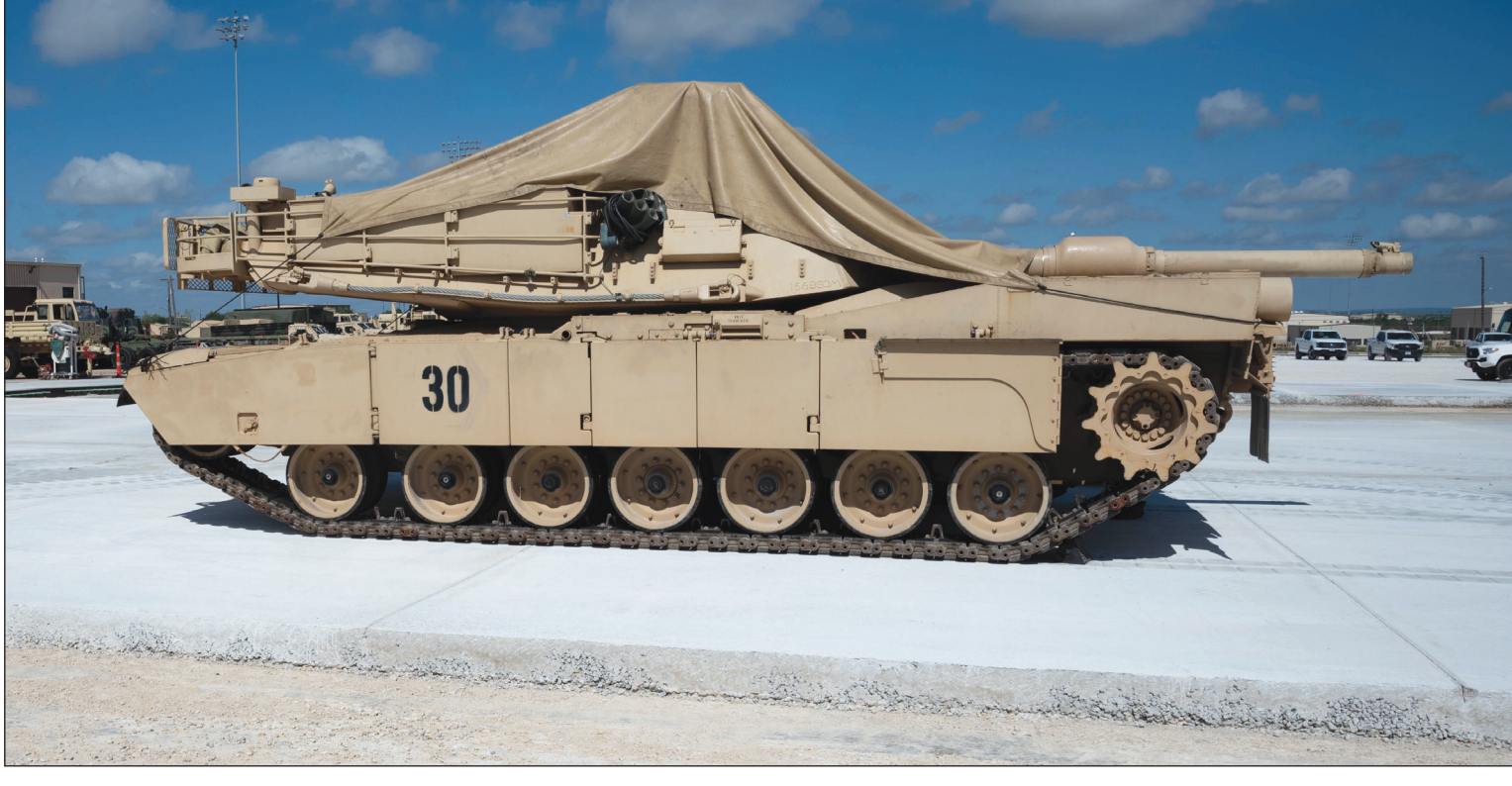
An Abrams M1A2 SEPv3 sits atop a recently finished roller-compacted concrete slab. RCC pavement can often be opened for heavy traffic 24-48 hours after placement, an advantage for use in many applications.
